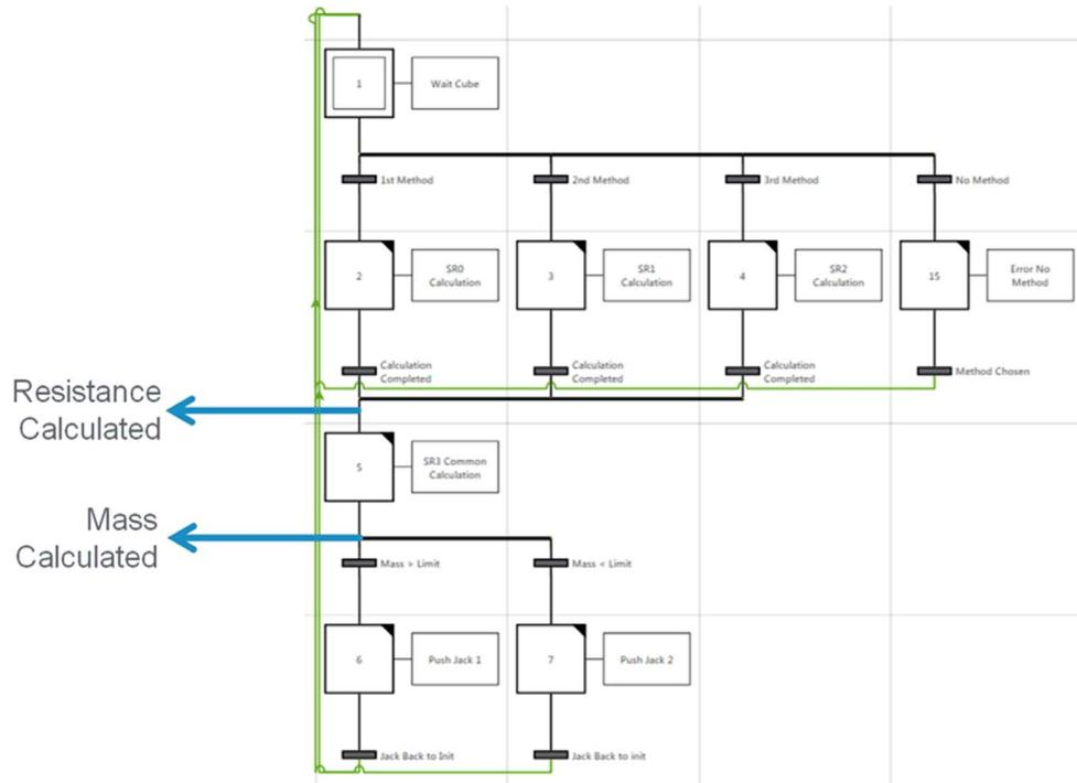
Initially, the machine is in the first step and jumps directly to step 15. This is the error state when there is no method selected and the signal light is red. As described in Setup Description ([see page 18](#)), the red signal light is mapped to digital output %Q0.6.
