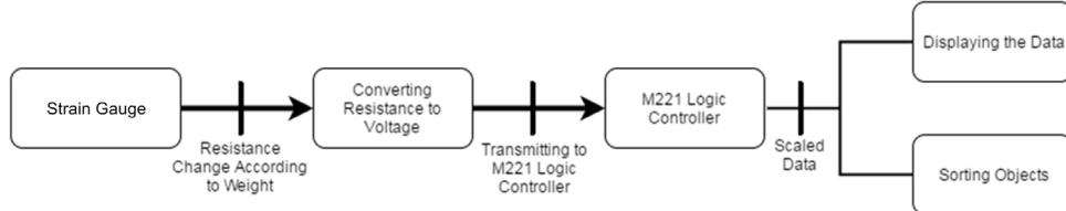
A strain gauge in a weighing scale measures physical data, the mass, by its changing resistance. The resistance is then converted to an electrical quantity (electrical potential).
