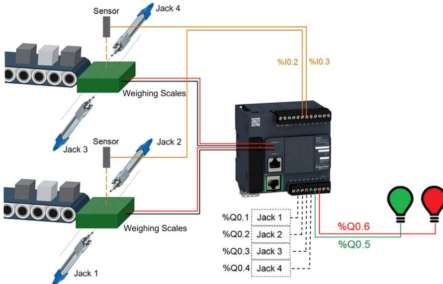
There are two weighing scales for sorting small boxes arriving from two conveyor belts. Depending on its mass, the pneumatic jacks push each small box right or left into larger boxes. The conveyor belts and the larger boxes are not in the scope of this example template.
